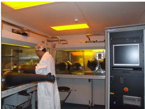
Figure 2 Nitrogen glovebox with incorporated organic evaporator and spin-coater
