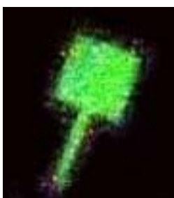
Figure 3 Enlarged view of a working OLED. The device was only 1 mm x 1 mm in size and was a prototype for display applications.
