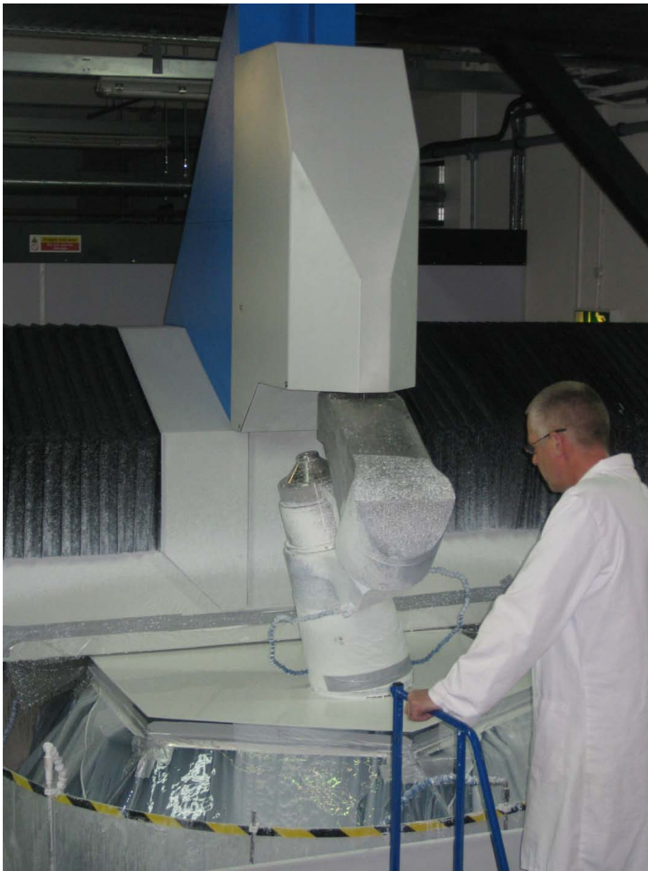
Master Segment in polishing at OpTIC
